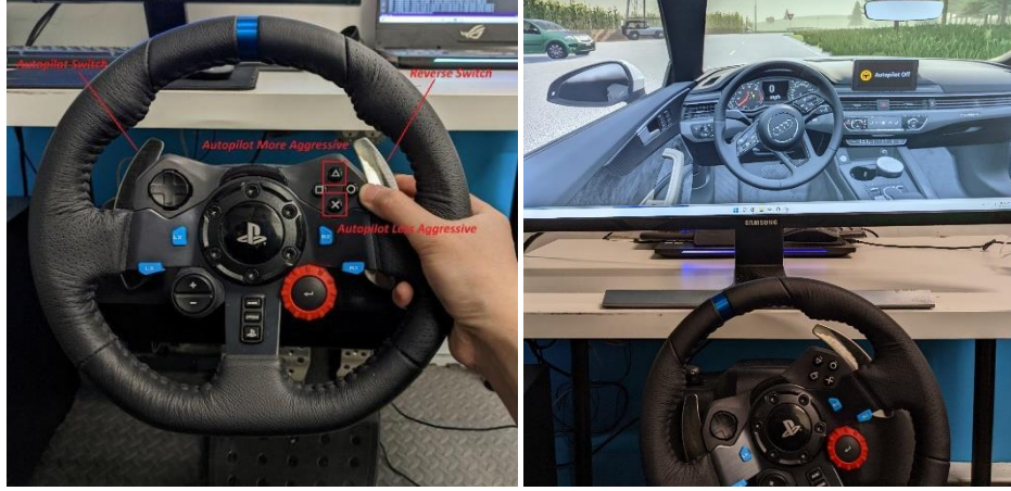
Fig. 3. Left: functions for buttons and switches. Right: physical and simulation wheel correspondence.
