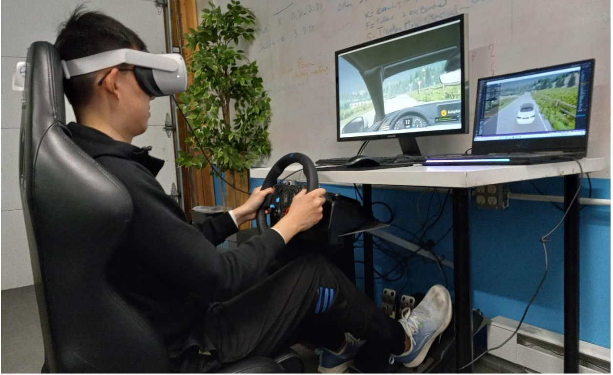
Fig. 8. Simulator demonstration: left monitor shows Carla server first person driver's seat view; right monitor shows the Carla client third-person tracking view.
